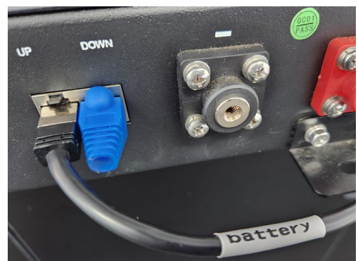
Fig. 3 - CAN Terminator in DOWN port
