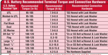
Proper connection is to position a lock washer between the nut and the connector (never between the connector and lead terminal) and apply the recommended torque or rough torque to completely compress the lock washer without deforming the lead terminal.
