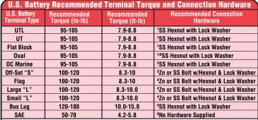
Proper connection is to position a lock washer between the nut and the connector (never between the connector and lead terminal) and apply the recommended torque or ough torque to completely compress the lock washer without deforming the lead terminal
